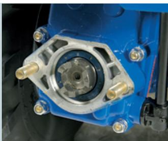
**POWER TAKEOFF** Independent power take-off with maintenance-free coupling in oil bath.
