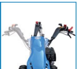
**1 Quick reverser** can be used without touching the gear shift lever.
