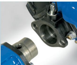
**QUICK COUPLERS** for replacing implements easily and quickly.
